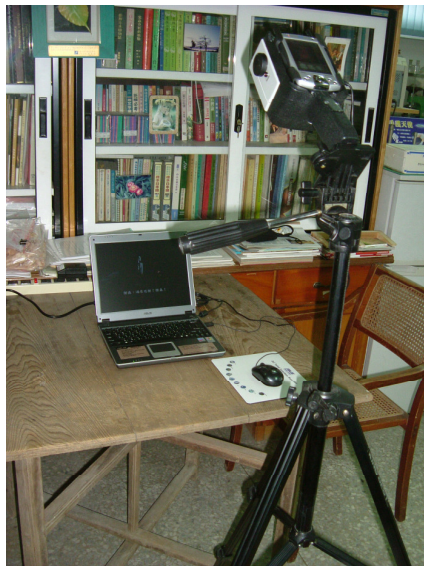
Figure 12 The setup situation for testing the laptop temperature
